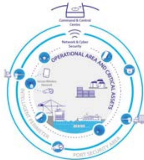
Figure 12: SAURON physical-cyber security architecture 60
